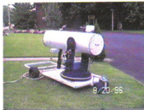
Figure 1 16" Newtonian telescope mounted on Scope Transport Unit.
